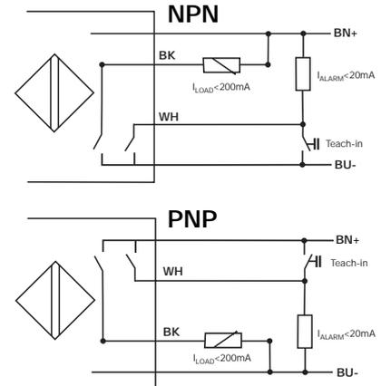
By means of the Teach-in wire, the functions described in the Teach-in Guide can be setup.
